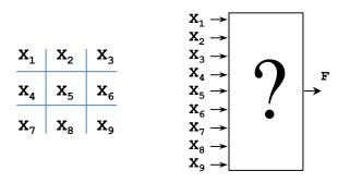
$\checkmark$  Sketch the logical circuit resulting from the Boolean equation for **F**.
