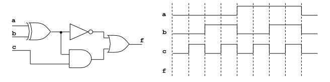
d) Complete the timing diagram of the logic circuit whose VHDL description is shown below: (5 pts)
